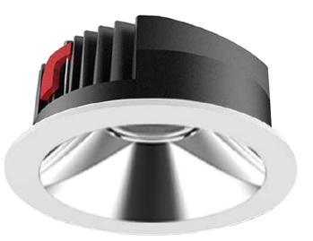
The Draco Max LED is a 226mm diameter downlight which uses a Cree XP-E LED array. The heatsink is constructed from die-cast aluminium complete with aluminium bezel and polished reflector. The downlight is available in outputs from 2550lm to 4250lm and as standard is rated IP20.
