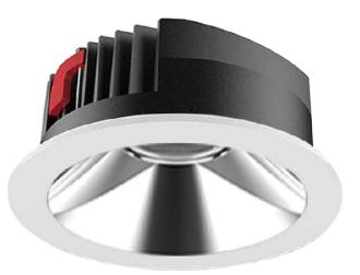
The Draco mini LED is a 182mm diameter downlight which uses a Cree XP-E LED array. The heatsink is constructed from die-cast aluminium complete with aluminium bezel and polished reflector. The downlight is available in outputs from 1700lm to 3400lm and as standard is rated IP20.
