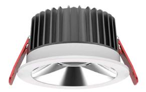
The Draco Mini LED is a 144mm diameter downlight which uses a Cree XP-E LED Array. The heatsink is constructed from die-cast aluminium complete with aluminium bezel and reflector. The Downlight is available in outputs from 1300lm to 700lm and as a standard is rated IP20.
