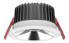
The Draco Nano LED is a 103mm diameter downlight which uses a Cree XP-E LED Array. The heatsink is constructed from die-cast aluminium complete with aluminium bezel and reflector. The downlight is available with 780lm and as a Standard is rated IP20.
